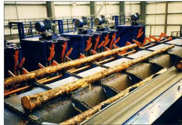
High capacity cross-cutting line for long poles
